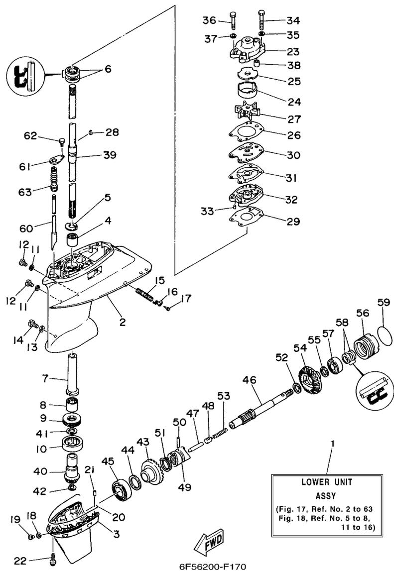
FIG. 17 LOWER CASING & DRIVE 1
